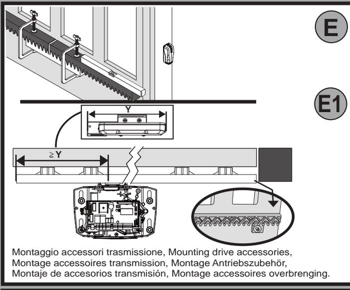
**Montaggio accessori trasmissione, Mounting drive accessories,
